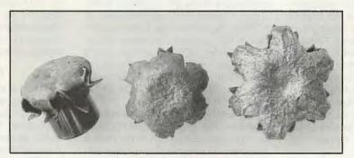
There are several requisites for pistol ammunition to have potential for physiologically incapacitating an aggressor: It must reliably penetrate to a depth to disrupt major organs and arteries; it must reliably expand to a dimension that leaves a large, permanent wound channel; it must stay in one piece so it can effectively cut tissue at the outer radius of the wound channel. Photo: Peter G. Kokalis
